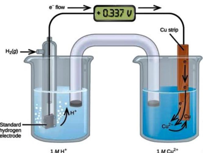
*i* → To calculate  $E_{\text{Cu}^{+2}/\text{Cu}}^\circ$ , make a cell  $\text{Pt(s)} \mid \text{H}_2(\text{g}) \text{ (1 bar)} \mid \text{H}^+(\text{aq.}) \text{ 1M} \parallel \text{Cu}^{+2}(\text{aq.}) \text{ 1M} \mid \text{Cu}$
